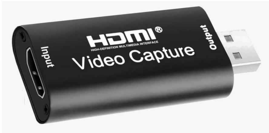
Connect the video capture card to your computer's USB port, and then connect the it with the analog DVR/camera via HDMI. If the DVR/camera does not support HDMI, e.g. if it supports S-video or VGA, then you can order a video capture card that supports S-video/VGA, or an S-video/VGA-to-HDMI converter.
